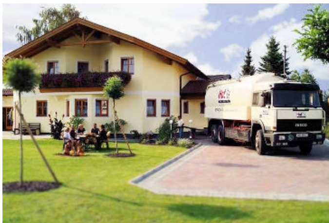
Fig. 11.1 Example of wood pellet delivery by pump-tank car (By courtesy of Glechner GesmbH Ko KG).
